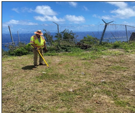
An ordnance and explosives safety specialist confirms response of emplaced QA seed item.
